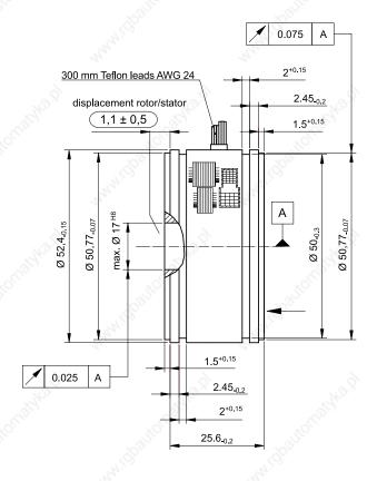
Inner diameter stator = 33.470 min. Outer diameter rotor = 32.735 max.
